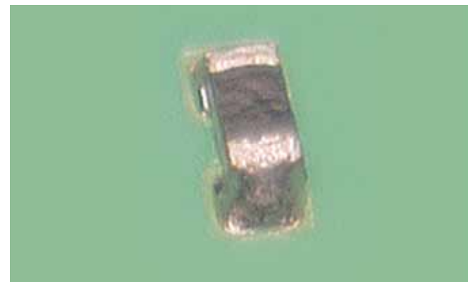
Microchip size 0201 which was soldered with a conventional paste; negative wetting angle, serious graping problems
